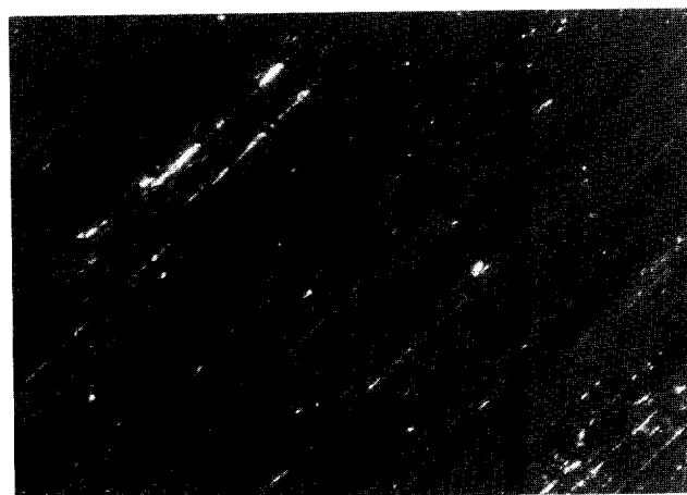
Figure 6 Microscopic photograph of P- p -H film on oriented poly( p -phenylene) under crossed nicols conditions. Thin film was cast from a chloroform solution
